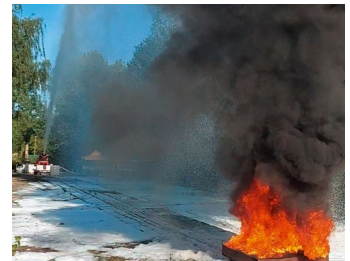
Fire tests for kerosene liquid fires were conducted and documented under the direction and supervision of FlameCert.
